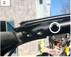
Re-torque all the fasteners after 100 miles.
